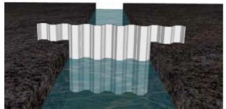
5. Where drains are greater than 1.5m and the weight of the water 6. could cause failure reinforcement should be added in the form of 10cm diameter vertical timber posts inserted into plastic piles (where Multi-lock is used) and support timbers fixed immediately behind the dam.
