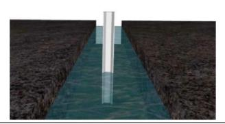
Push the first pile into the centre of the drain and drive using slow 2. short bursts of pressure from the excavator bucket or a rubber mallet until secure. (If necessary, protect the top of the plastic using a timber batten.) Please ensure that the pile remains vertical and is embedded 75cm below the invert of the drain.
