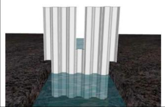
Drive piles into the final position starting with the centre pile until all 4. piles are approximately 30cm above the level of the surface.
