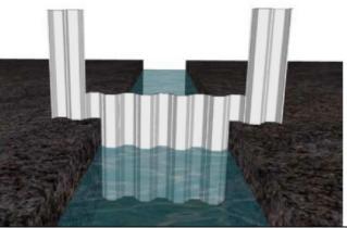
The dam should extend beyond the width of the drain into the bog, typically by a minimum of 75cm to prevent water from flowing around the dam and eroding the sides of the drain. Drive all piles to the final position.
