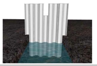
Guide adjacent piles into position, again use a machine bucket or rubber mallet to drive into a firm vertical position ensuring they are embedded at least 75cm below the base of the drain until the plastic is held secure.
